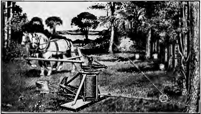
Fig. 29. Capstan Horse-Power Puller Made by Faultless Stump Puller Co., Cresco, Iowa
